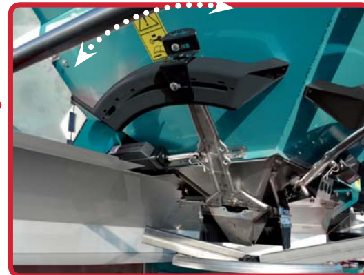
Electric setting from the cab (ECONOV version)
