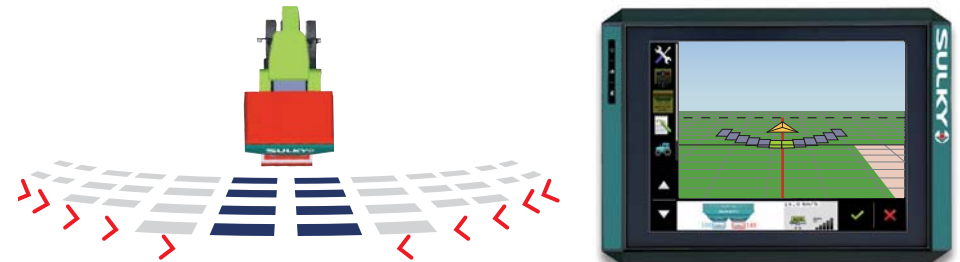
In a straight headland, before the complete closure of the distribution area, only the 2 centre sections remain open... so the accuracy of spreading in a curve is maximal.
