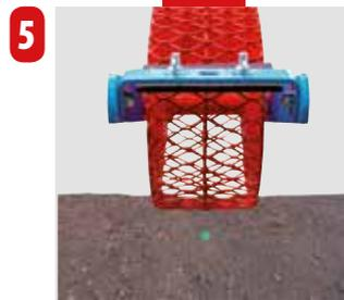
5) The rear wheel closes the furrow around the seed for optimal seed germination.
