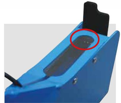
The monitor sensors are placed under the metering boxes, inside the shoes. A light beam checks the seed passage, even the smallest of seeds.
