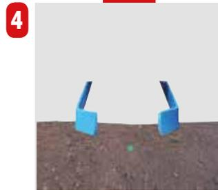
4) The scrapers\* (retractable if necessary) scrape fine soil over the seeds.
