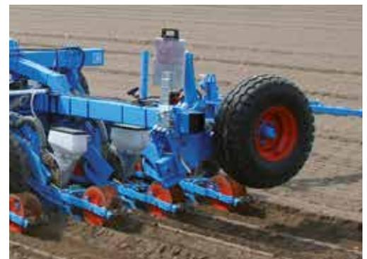
A lengthways transport carriage is available for wide-configuration planters. This transport carriage has a manual or hydraulic wheel lift.
