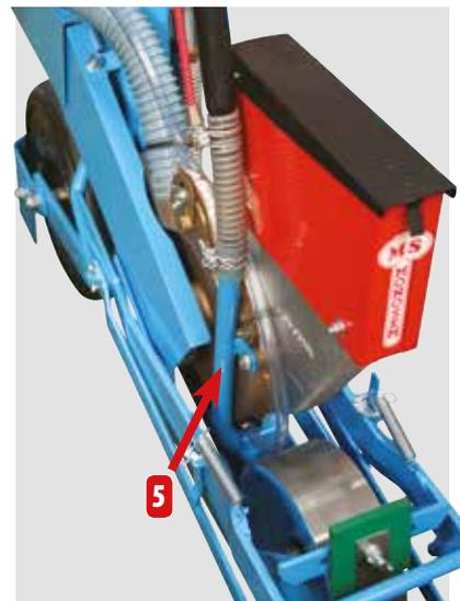
The insecticide Microsem tube (5) is placed just behind the shoe so as to distribute the product in the planting line.
