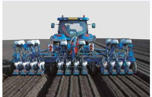
MS D2 Planter - Double bar folding frame - 3 x 4 double rows with Microsem
