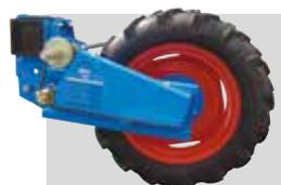
Adjustable wheel unit with 500 x 15 wheel and integrated metering box
