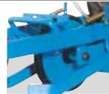
Intermediate press wheel with self-cleaning supple tyre
