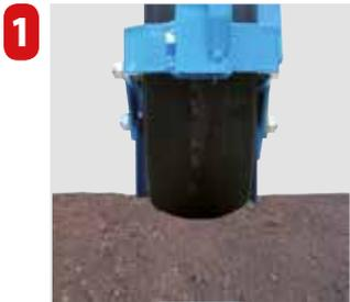
1) The clod remover clears the future planting line of clods or stones whilst the gauge wheel presses the soil and controls the depth.
