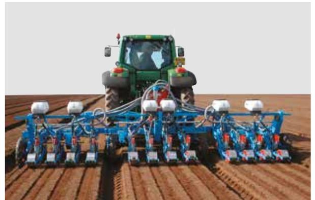
MS C Planter - Double bar folding frame - 3 x 4 rows with Microsem
