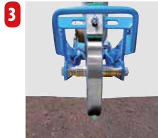
3) The intermediate press wheel\*, adjustable in pressure, presses down the seeds into the bottom of the furrow for regular and rapid plant emergence.
