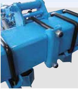
The assembly of the units with clamps ensures a reliable and solid fixing of the units. If necessary, the units can be moved in order to modify the inter row spacing by loosening the clamps. This method of fixing excludes the risk of the metering unit sliding sideways when working.
