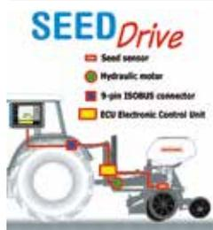
The SeedDrive hydraulic control of the seed population replaces the planter seed spacing gearbox(es) by several hydraulic motors which drive the seed discs. This system offers the possibility of non-stop modulating of the seed population directly from the tractor cab with the TOUCH Mini or TOUCH terminal or another ISOBUS compatible terminal.
