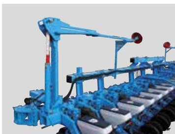
The hydraulic row markers for rigid and coupled frames are single, double or triple folding according to the width of the planter (see above, row marker for 18-row rigid frame).
