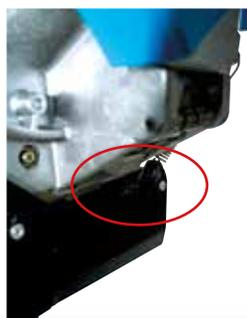
The seed monitor sensors are placed under the metering boxes, inside the shoes. A beam of light enables the control of the seed passage, even the smallest seeds.
