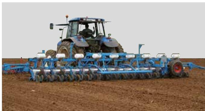
18-row rigid triple bar MECA V4 planter with Microsem and transport carriage
