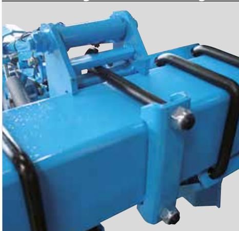
The metering unit fixing system by clamps enables sure and solid fixing of the metering units. If necessary the metering units can be moved so as to modify the inter row spacings by loosening the clamps. This system of fixing excludes all risks of lateral movement of the metering units during work and resists in the most difficult operating conditions.
