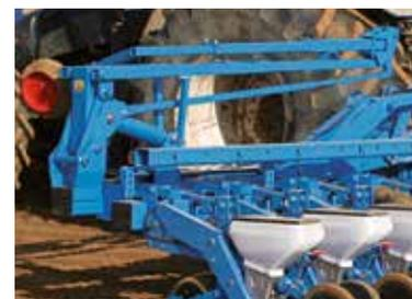
The hydraulic row markers for folding frames are equipped with a compact folding system (see above, row marker on 3-level folding frame).
