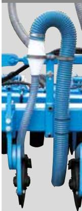
The cyclones assembled opposite each metering unit allowing the fertilizer drop by gravity and thus limiting the dust forming due to the pulsed air.
