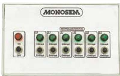
The electromagnetic row cut-off systems with manual control enable an individual declutching of each metering unit from the tractor cab. Each row is equipped with a rotation control light. This system is available in 2, 4, 6, 8 and 12 rows.
