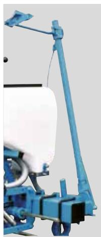
In the standard version, the 6-row planters are equipped with manual row markers with shoes. Hydraulic row markers with discs are available on option.
